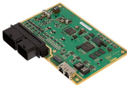
Audi's zFAS central driver assistance controller.
