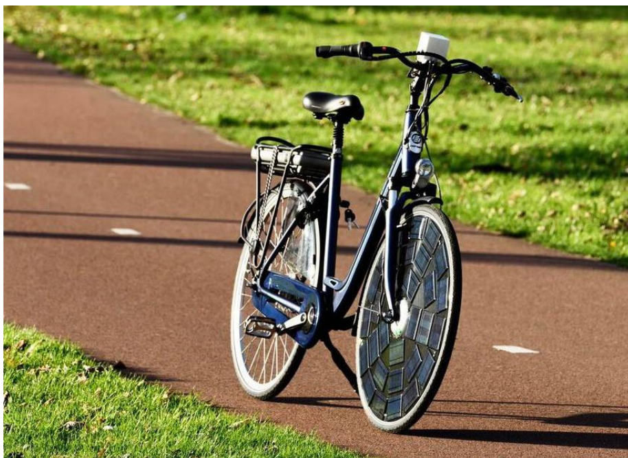
Solar Application Lab's first prototype sports 60 mini solar panels on its front wheel and a hub-mounted electric powertrain.
